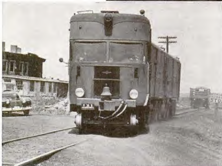
Leaving the rails, this train will roll along on 42 rubber-tired wheels
